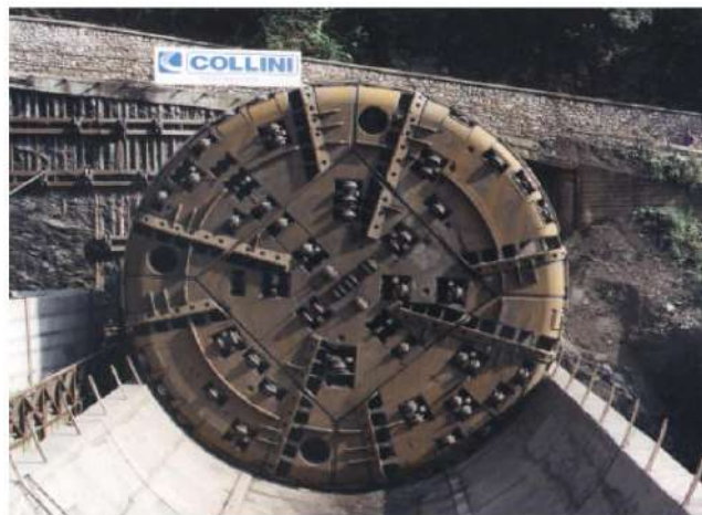
Figure 2.21: Tunnel Boring Machine
