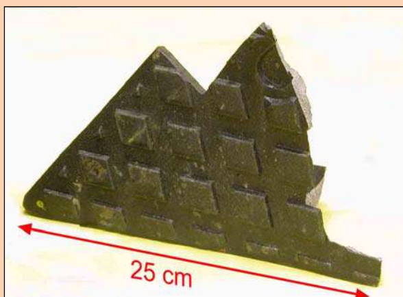
Figure J.1: Portion of a manhole covering broken in the load bearing capacity test ( \geq 400 KN )
