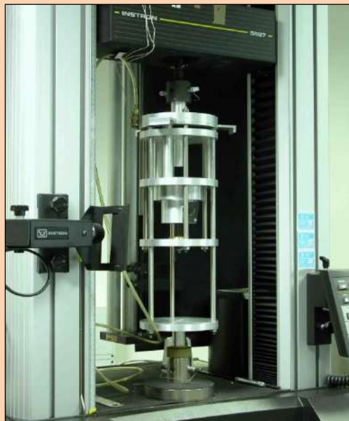
Figure J.4: Dynamometer attachment to measure bursting strength
