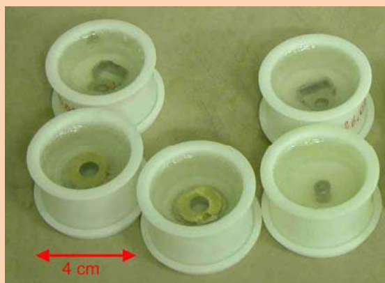
Figure J.2: Specimens mounted in thermosetting epoxy resin
