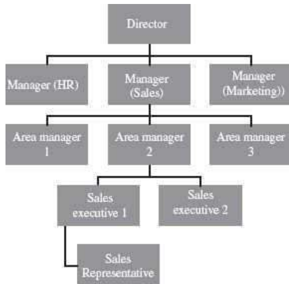
Figure 12.7 Hierarchical database model
